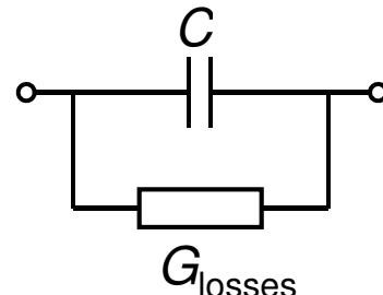
$$\begin{aligned}\underline{Y}_{real} &= G_{losses} + jB \\ &= G_{losses} + j\omega C\end{aligned}$$
