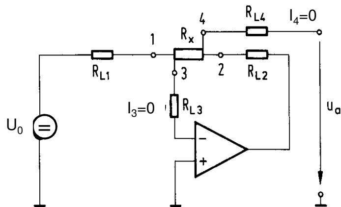
4-Wires-connection and constant current supply
