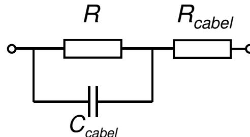
$$\underline{Z} = R_{cable} + R \parallel j\omega C_{cable}$$
